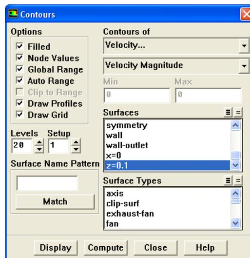
(a) Select Velocity... and Velocity Magnitude from the Contours of drop-down lists.
