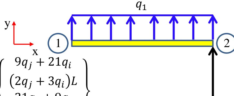
$$\{f_e\} = \begin{Bmatrix} T_i \\ M_i \\ T_j \\ M_j \end{Bmatrix} = \frac{L}{60} \begin{Bmatrix} 9q_j + 21q_i \\ (2q_j + 3q_i)L \\ 21q_j + 9q_i \\ -(3q_j + 2q_i)L \end{Bmatrix}$$
