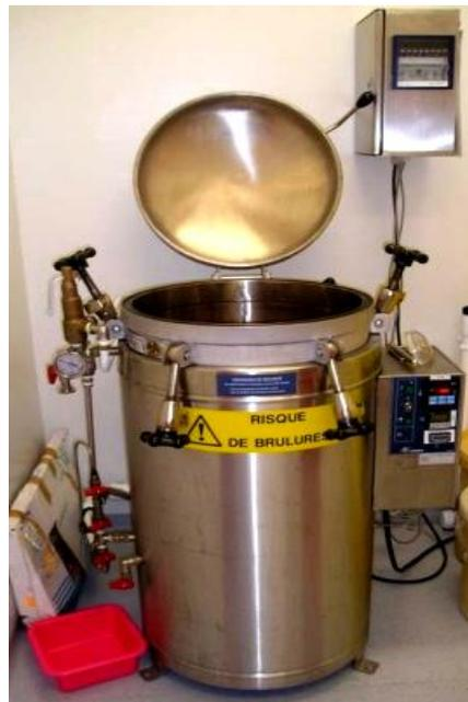
**Fig.25** Autoclave. (Source : <https://www.laboratorydeal.com/products/laboratory-vertical-autoclave-98-liters>).
