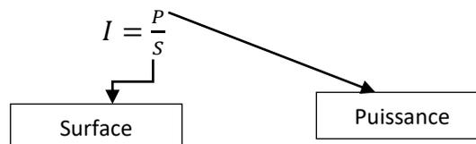
$$[I] = \frac{[P]}{[S]} = \frac{\text{Kg} \cdot \text{m}^2 \cdot \text{s}^{-3}}{\text{m}^2} = \text{Kg} \cdot \text{s}^{-3}$$
