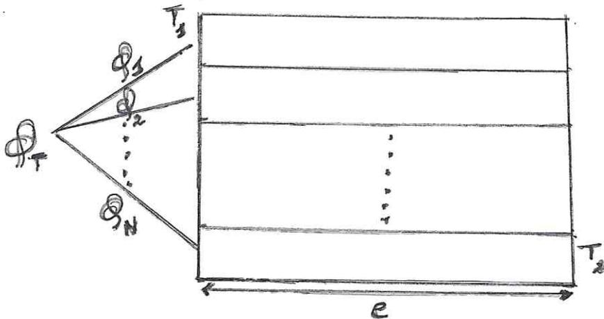
$$Q_1 = \frac{T_1 - T_2}{R_1}, Q_2 = \frac{T_1 - T_2}{R_2}, \dots, Q_N = \frac{T_1 - T_2}{R_N}$$
