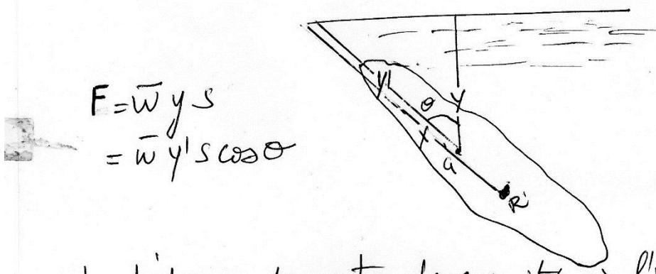
$$\begin{aligned} F &= \bar{w} y s \\ &= \bar{w} y' s \cos \alpha \end{aligned}$$
