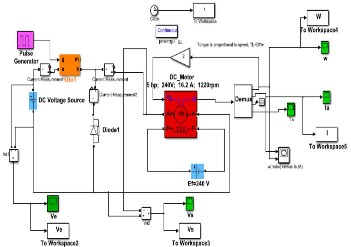
Block Parameters: DC\_Motor 5 hp; 240V; 16.2 A; 1220rpm
