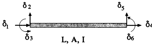
Figure 3-6 Positive displacements for the frame elements.
