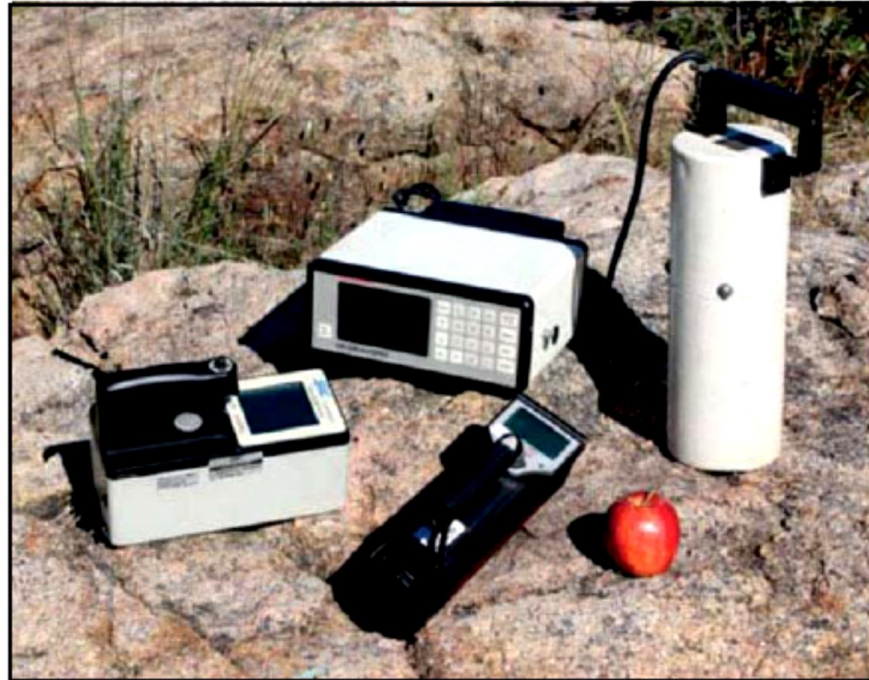
Figure 4.8 Examples of modern \gamma -ray spectrometers. Exploranium GR-320 enviSPEC with large external sensor (rear); Exploranium GR-135 miniSPEC (front left); Radiation Solutions RS-125 Super-Spec (front right).
