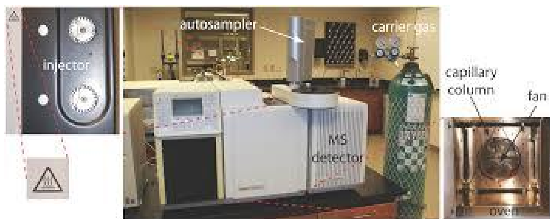
Figure 2.5 Gas chromatography.
